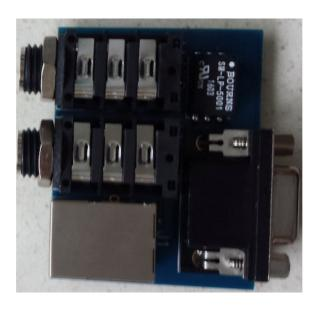
Connecting the TMC-1 to the I-Mon using a pair of RJ45 breakout boxes
